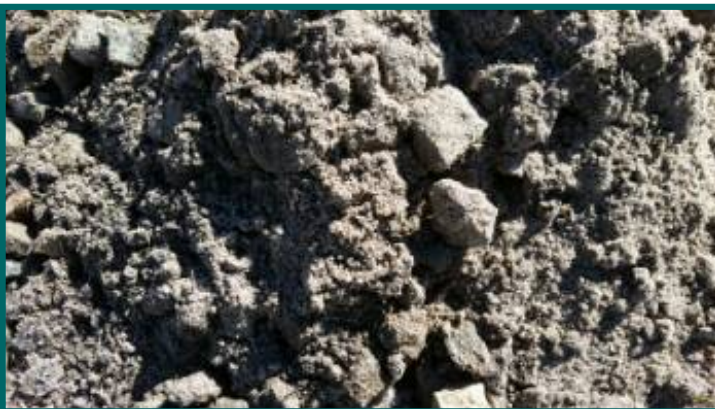
Leach field sand and stone.
